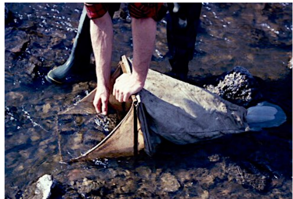
Figure 14: Kick net sampling (left) and surber sampling (right) aquatic macroinvertebrates
